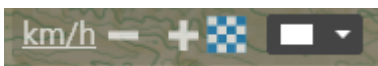
Figure 29: Graph control Buttons (Unit Type, Zoom Out, Zoom In, Change Opacity, Change Text Colour)
